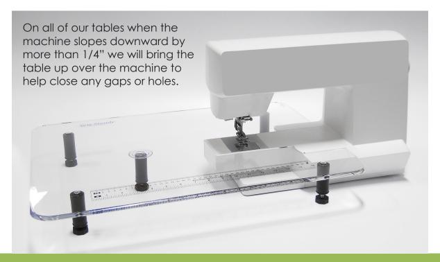
It is very important to have the entire table flush and level with the top of the free arm at the needle, so it is important to have the legs on the table for proper fitting. If the table is even 1/8" lower than this point it can cause the table to hit the machine and lift up on the right side.
