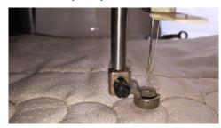
Important: The Ruler Foot is higher than standard feet and therefore you cannot lower the needle when the foot is raised. When using the Ruler Foot we advise that you turn on your machine with foot lowered.
