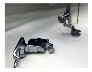
Lower the shank and place the Ruler Foot on the shank, replace the screw.
