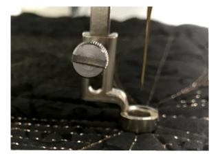
Place the quilt sandwich under the Ruler Foot with the screw just loose.
