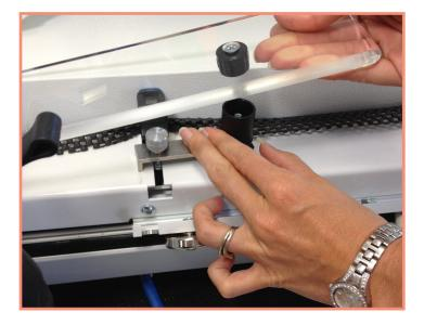
Step 4: Tighten the thumb screw under the carriage to secure bracket to the carriage.
